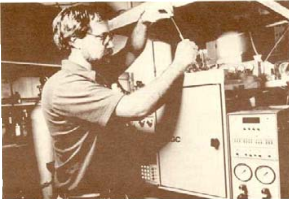
Bodega Marine Lab manager, Paul Siri, injects a small test sample into one of the lab's gas chromatographs. The lab shown here will be used to analyse extracts of sediment and tissue samples for oil pollutants.
